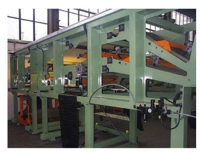
constant material tension during the various stages of application. Any spiral winding patterns can be programmed into the machine recipes.
