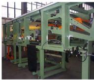
with Allen Bradley or Siemens PLC components. A touchscreen MMI is provided as standard, with graphic interface and dedicated screens for every machine function, recipe management, alarm handling and production statistics.
