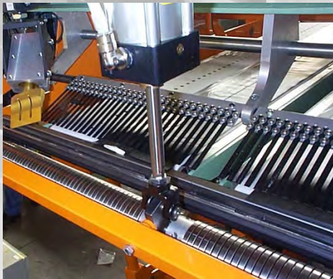
Sidewalls Servicers with ultra-sonic cutting
